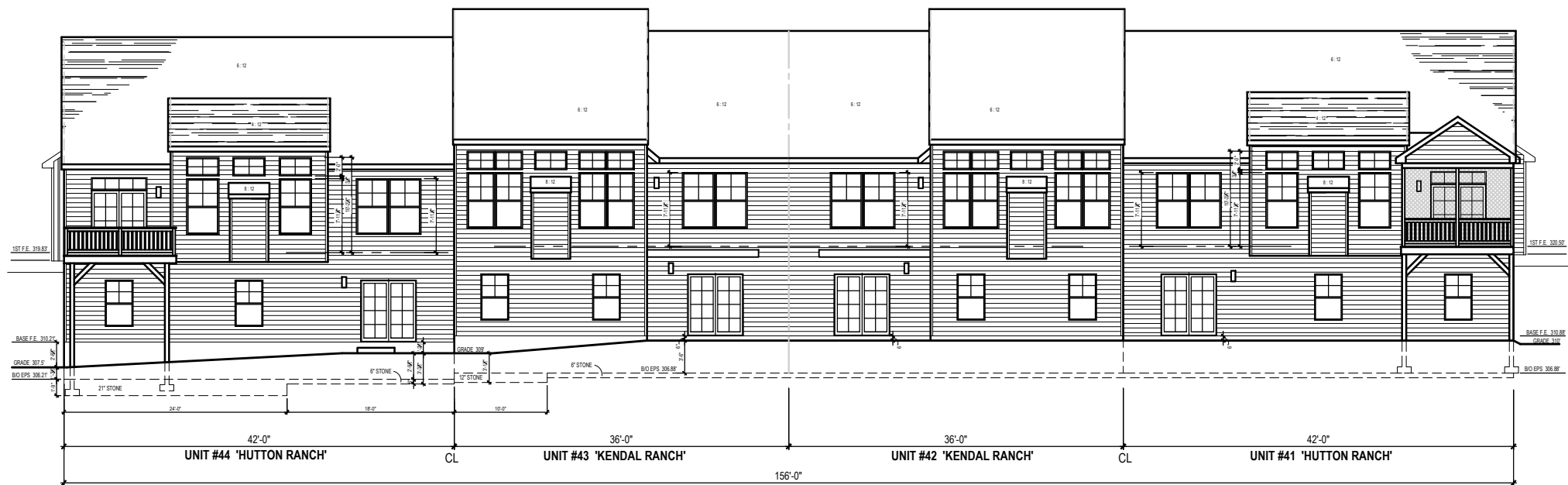
2 OVERALL REAR ELEVATION A104 SCALE: 1/16" = 1'-0" SEE ALSO ENLARGED INDIVIDUAL UNIT PLANS
